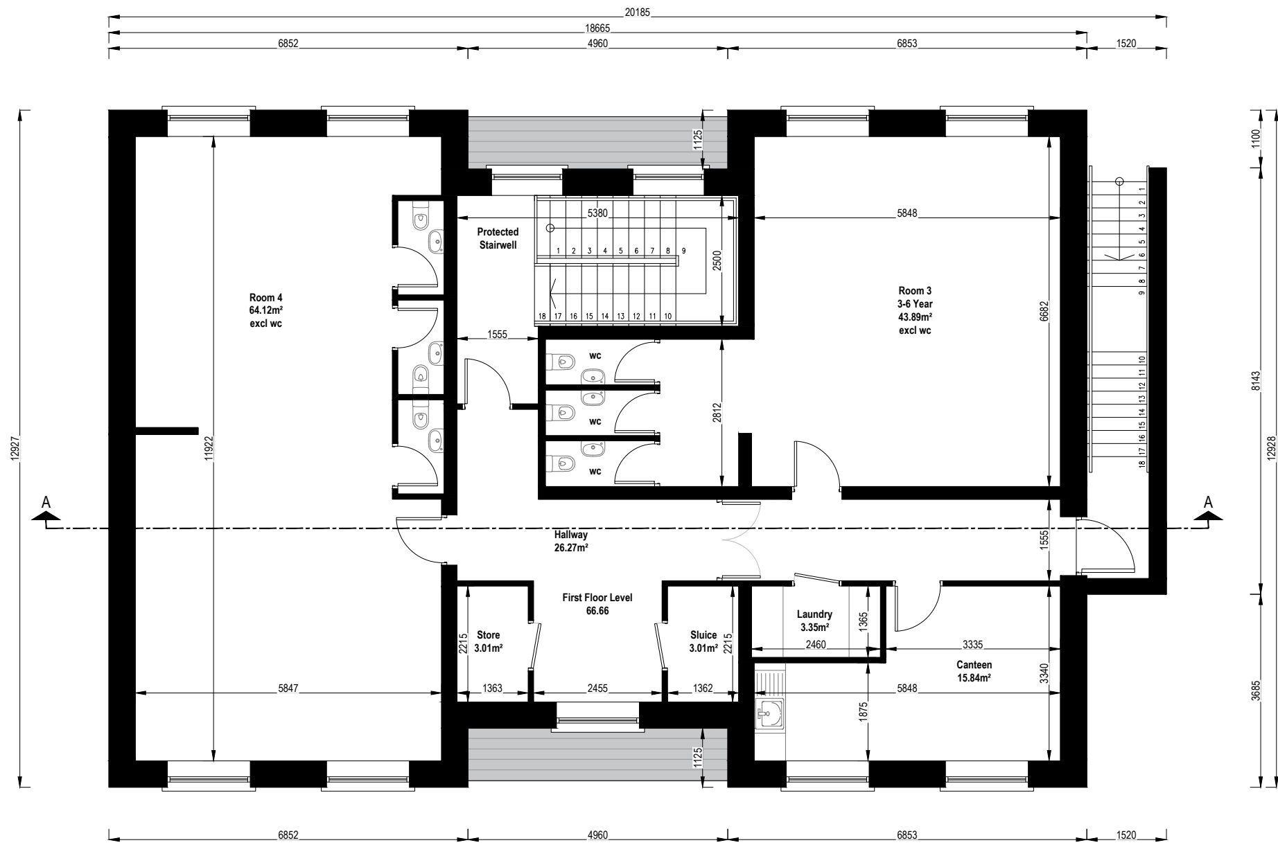
FIRST FLOOR PLAN Scale 1:100 First Floor Area 197.13m 2 Total Floor Area 394.26m 2
